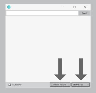
After flashing the Arduino with the code below, open the serial monitor and set it to append *carriage return* only and then set the baud rate to 9600.
