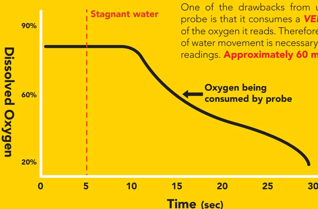
One of the drawbacks from using a galvanic probe is that it consumes a **VERY** small amount of the oxygen it reads. Therefore, a small amount of water movement is necessary to take accurate readings. **Approximately 60 ml/min**.
