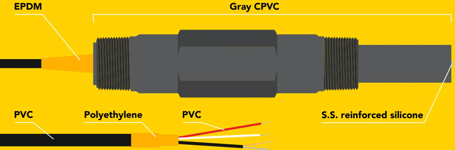
**This Dissolved Oxygen probe can be *fully submerged* in fresh or salt water, up to the Tinned leads *indefinitely*.**
