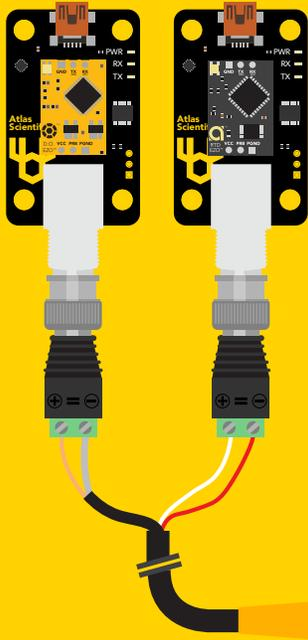
Using two **BNC with Terminal Screws**, you can easily connect the Industrial Dissolved Oxygen probe to our **EZO™ D.O. Circuit** and **EZO™ RTD Circuit** via our **Electrically Isolated USB EZO™ Carrier Board**.
