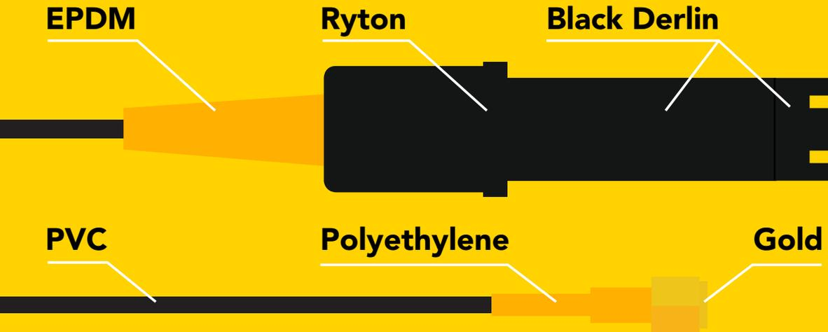
**This Mini Dissolved Oxygen probe can be *fully submerged* in fresh or salt water, up to the SMA connector *indefinitely*.**
